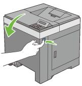
4 Open the belt unit until it stops and remove the jammed paper. Confirm that there are no scraps of paper remaining inside the printer.
